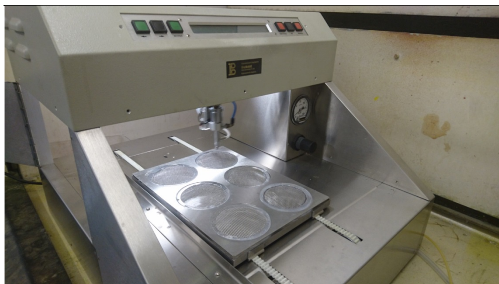
Figure 10.2.1. Burkard computer controlled bench top sprayer, griddled lids used to contain weevils in petri dish whilst applying spray treatment
